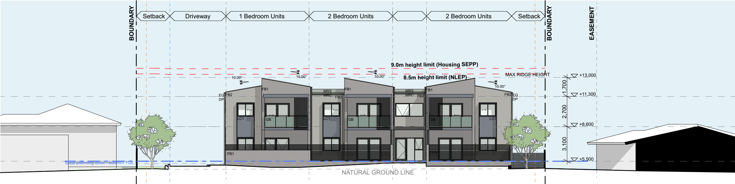
2 North Elevation (Building B) SCALE 1:200 @ A3
